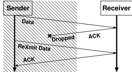
Figure 3: Receiver incorrectly assumes (shaded region) that probes are valid retransmissions from sender due to lost ACK.
