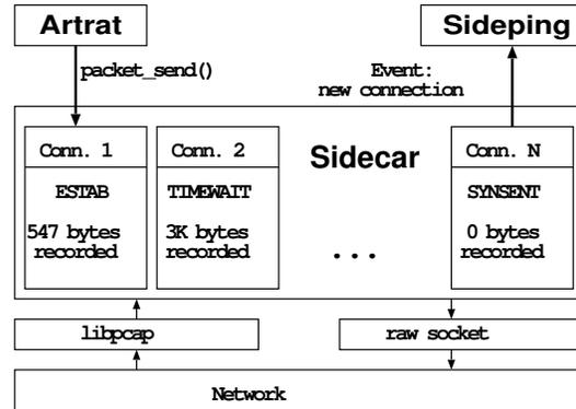
Figure 1: Sidecar is a platform for unobtrusive measurements that provides an event-driven interface and connection tracking to higher-level tools, e.g., artrat, sideping.
