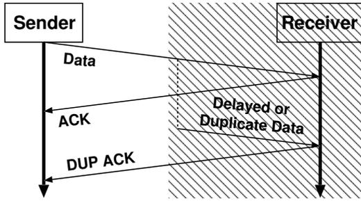
Figure 2: Sender incorrectly assumes (shaded region) that duplicate ACKs are from delayed, reordered, or duplicated packets.
