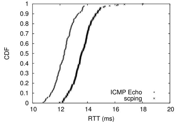
Figure 6: Sideping RTTs vs ICMP Echo: Difference exposes NAT + wireless network.
