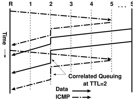
Figure 7: Overview: Artrat correlates congestion and queuing delays to do receiver-side bottleneck location (example: bottleneck from S to R at TTL=2).
