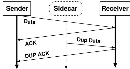
Figure 4: Reality: Sidecar probes are replayed data packet that generate duplicate ACKs. Probes are transparent to both sender and receiver applications.
